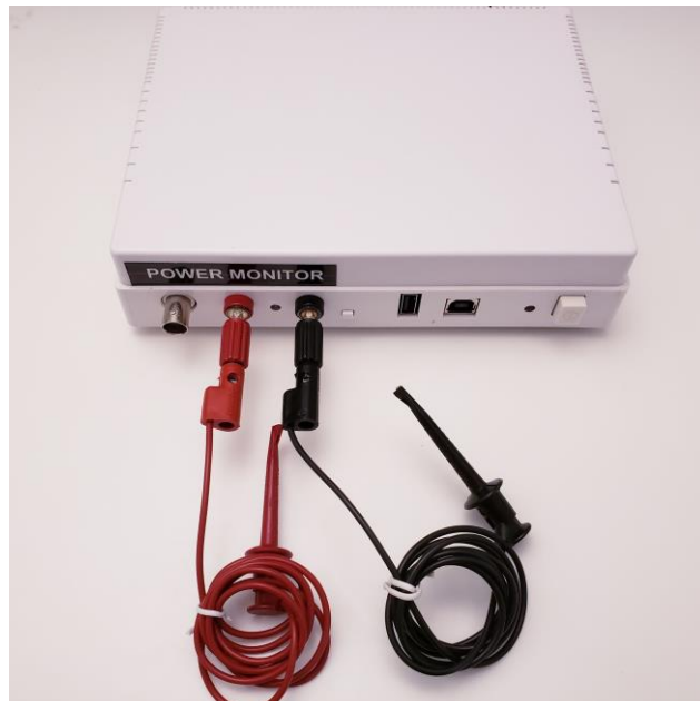
Figure 26. Monsoon Power Monitor Hardware
